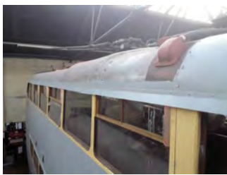
The offside of Cardiff 262 showing the longitudinal rainwater deflector strips above the windows of both decks.
