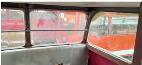
The completed front offside upper deck hardwood window surrounds on Cardiff 262.
